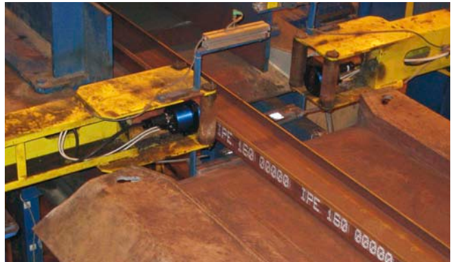
Marking of H-beams
