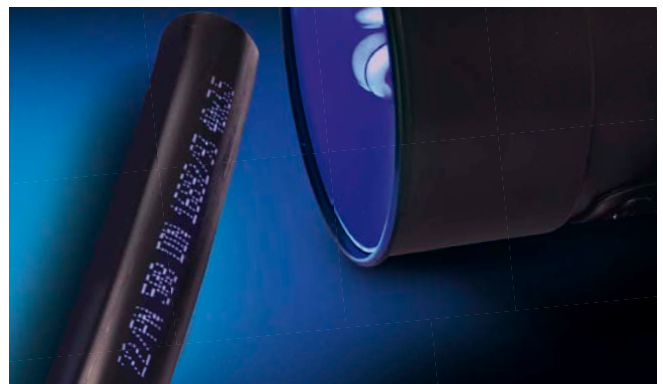
Marking of plastic pipes with UV ink
