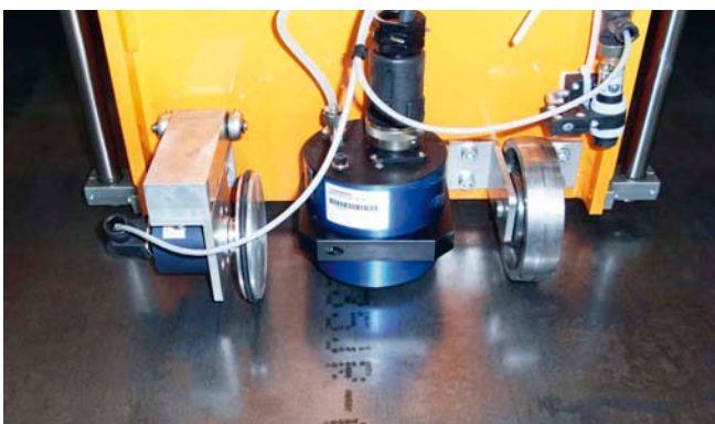
Steel sheet marking with etching ink
