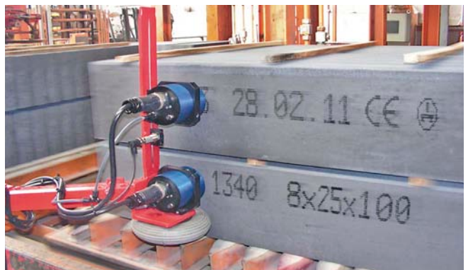
Coding of precast concrete elements
